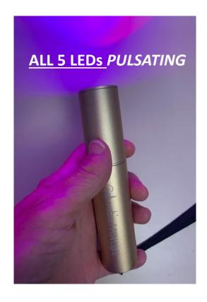
Press the button once and release. Then hold the button down for 3-5 seconds until it flickers and release. You are now on the **pulsating mode** with all 5 of the LEDs on
